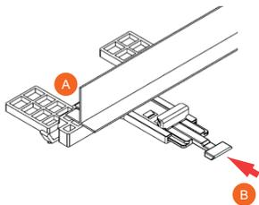
**Note:** For clarity, [Figure 2](#) only shows the T-bar bracket and the T-bar, and does not show the R700 AP.
